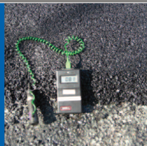
Compaction temperature of Life 10 mm CGSC (T 81 0C)
