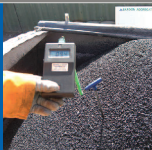
Temperature of Life 14 mm CGSC after discharge (T 94 0C)
